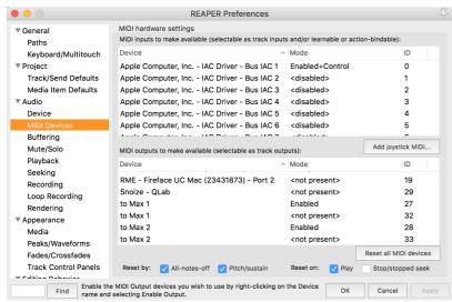
Then set the midi output of track 9 to 'to Max 1' (click the i/o button on the track). Select the track and open the 'item' 'source properties' menu. 'Send MIDI (MTC)' should be checked.
