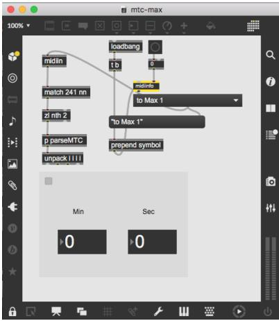
• in reaper configure the midi output 'to Max 1' for time code being sent to max.
