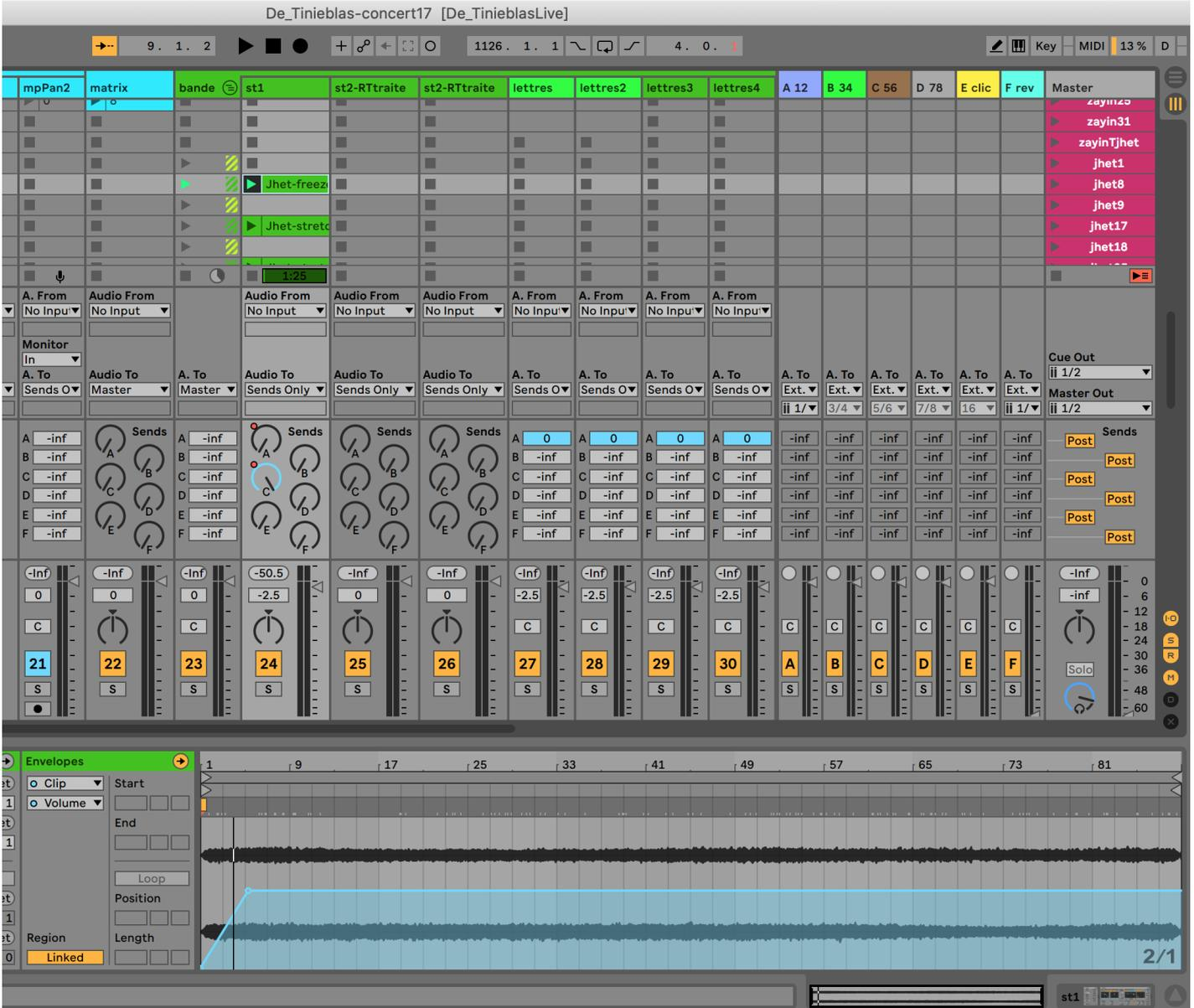
'st2-RTtraitements' is a track for soundfiles that can be processed by realtime treatments in their rack device.
