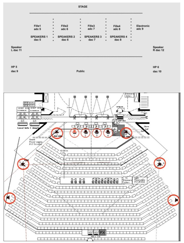
The speakers "L", "R", 5 and 6 are direct outputs from the computer dac~.
