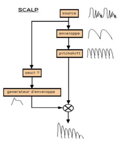
The scalp is an effect that transforms the actresses' voices into percussive sounds. The envelope of the four voices of the actresses is extracted and pitchshifted in order to create four different timbres. To these timbres, we allocate an envelope that is triggered according to a threshold of each voice. It is possible to switch from the normal voice to the transformed voice.
