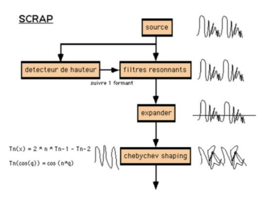
Scrap is an effect using non-linear distortion with transfer functions described by Chebycheff polynomials. This distortion keeps the harmonic components of harmonic sounds. By sending a sine of 100 Hz, a polynomial of order 5 would output a sine of 500 Hz. Starting from the source, the program tries to follow a formant and isolates it from the rest using a bank of resonant filters. The attacks are accentuated with an expander and distortion is applied to it later.
