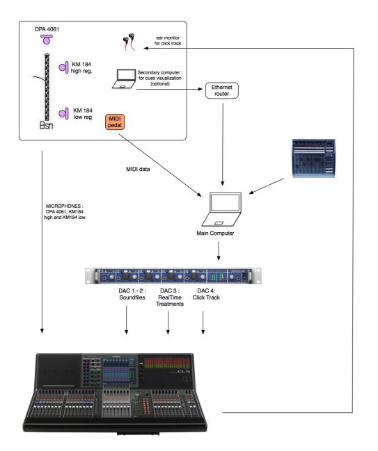
The sound files from the electronics are output from the audiocard through dac 1 + 2. The electronics can be also output in "cross Stereo" configuration (cross stereo: left channel is output from front left and rear right, while the right channel is output from front right and rear left). Treatments for the basson are output through dac 3
