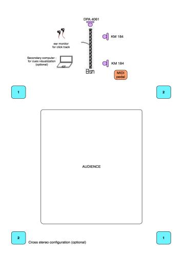
A DPA 4061 microphone is attached to the top of the instrument with an elastic, + two Neumann KM 184 microphones are used, in order to catch both registers of the instrument, corresponding to the position of the hands of the player.
