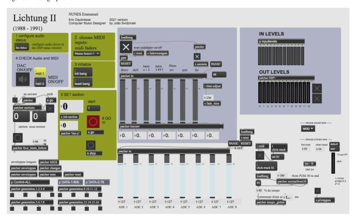
The DSP patch is accessible in the [patcher DSP~], at the left, just bellow "OUT LEVELS" The two control system are in the middle [DATA-1-80b] and [DATA-2-78].
