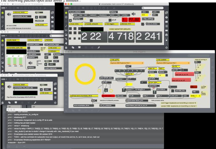
encantadas main score 10 paris: this is the patch controlling and distributing via OSC all the events. In the midi\_triggers subpatch the red message Kill\_exec\_proc is stopping all the running events. The midiconnect is patched as the following: sy77 and KX88 on USB1, BCF2000 on Host2, extra keyboard HST4)
