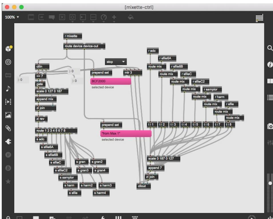
Midi controller #7 is used for the control faders :
