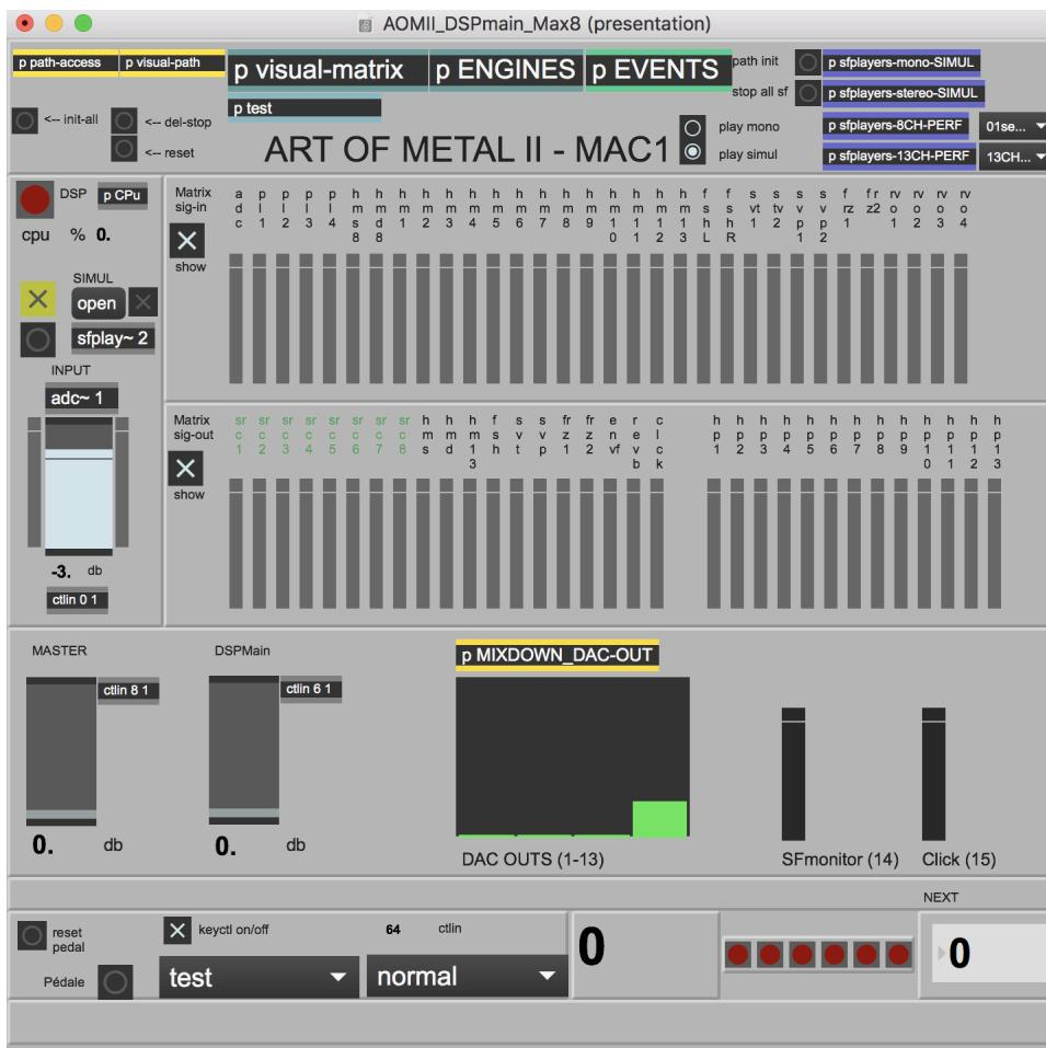
This patch handles the sound fx, the soundfiles, the score & transport. The Input levels, Fx levels and master out are followed here (by mici ccs). It is the main audio inputoutput. It sends and receives audio with the spat patch.
