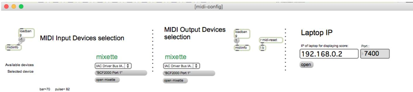
2. Click on '2-config' (figure 'midi-config') and select the midi input/output of 'mixette' in order to configure your MIDI setup for the control surface (for mixing of adc, sfiles, samplo, harm and gran). You can access the routing of midi channels by clicking on 'mixette' (see picture below).
