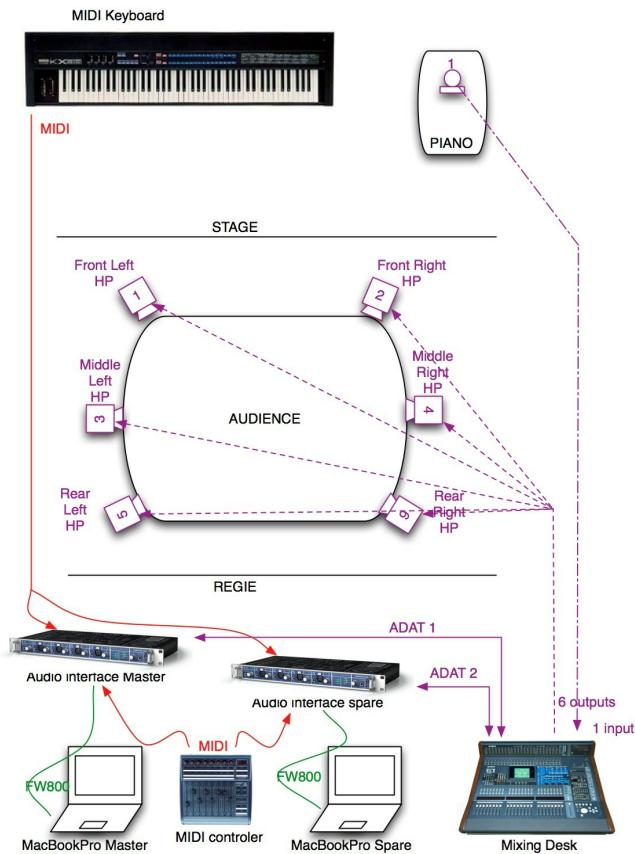
Audio from microphones are sent to computers through the mixing desk. The Master and Spare computer receive the same inputs. Only Piano needs microphones.
