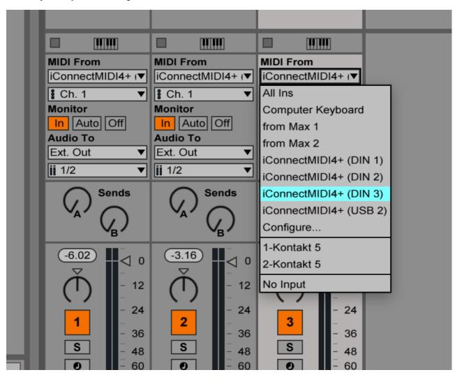
Please refer to the sound engineer stage setup for the connection of the midi keyboards. The 3 samplers should be set on 3 individual stereo outputs routed in the mixing desk with the Dante controller.
