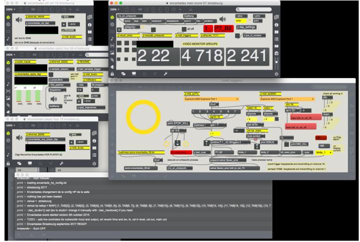
• *encantadas main score 10 paris* : this is the patch controlling and distributing via OSC all the events. In the midi\_triggers subpatch the red message **Kill\_exec\_proc** is stopping all the running events. The midiconnect is patched as the following : sy77 and KX88 on USB1, BCF2000 on Host2, extra keyboard HST4)
