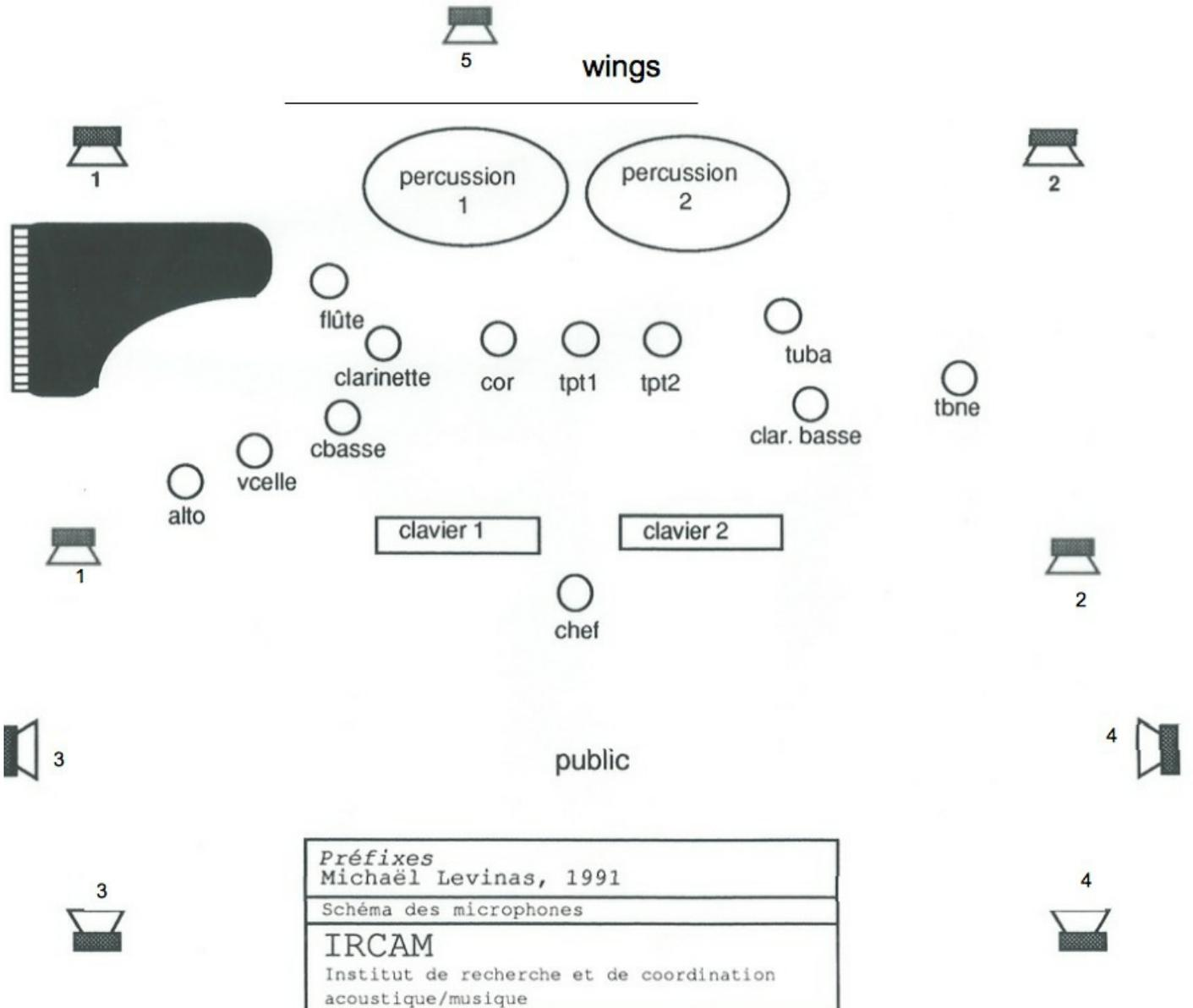
The loudspeaker "in the wings" can be in the wings if you can keep the door open. If you can't, you can put it under the audience or face to the back wall. What is important is that sounds from this loudspeaker seem to be far away from the audience.
