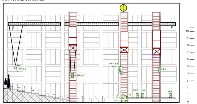
Essentially this configuration has 7 loudspeakers around the public (HP1 to HP 7 in the scheme), an 8<sup>th</sup> (preferably smaller) loudspeaker in a corner, turned towards the corner (HP8, referred as "Is solo" in the patch), two loudspeakers (9<sup>th</sup> and 10<sup>th</sup>, HP9 and HP10) have to be put within the ensemble, turned towards the public. A click-track for the conductor has to be planned.
