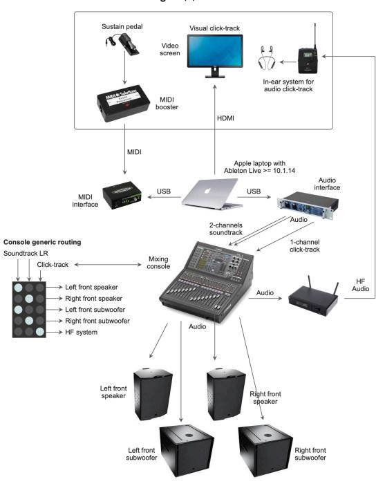
Stage Equipment for conductor
